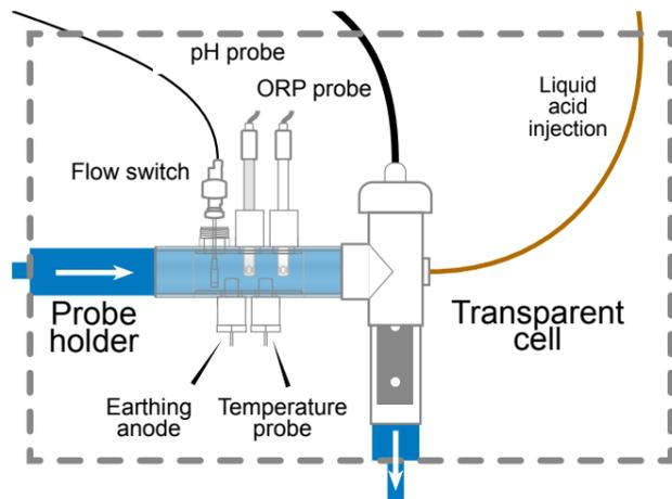
**Installation and connection of the cell (see diagram):**
