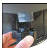
Sand easily accessible by removing the collar
